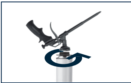
Turn gun on canister / turn straw on canister
