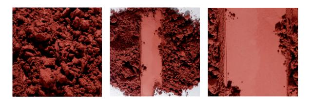
Two powder blends, both of the same shade. Right: Without titanium dioxide. Left: With titanium dioxide. The loose powder shows no visual colour difference. When smoothly pressed down it shows the higher luminosity of the titanium dioxide-free formula.
