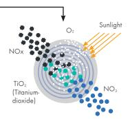
The catalyst titanium dioxide is not consumed. As long as the crystals are supplied with energy by electromagnetic waves (light), the process remains active.
